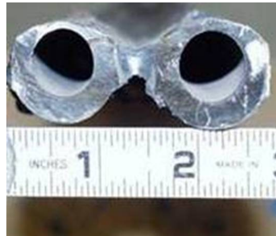
Photographs of waterwall and a cross-section of tubes showing the extent of corrosion and wall thickness wastage
